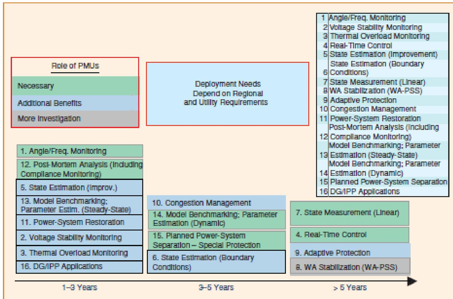
figure 10. Roadmap for deploying PMU applications.
