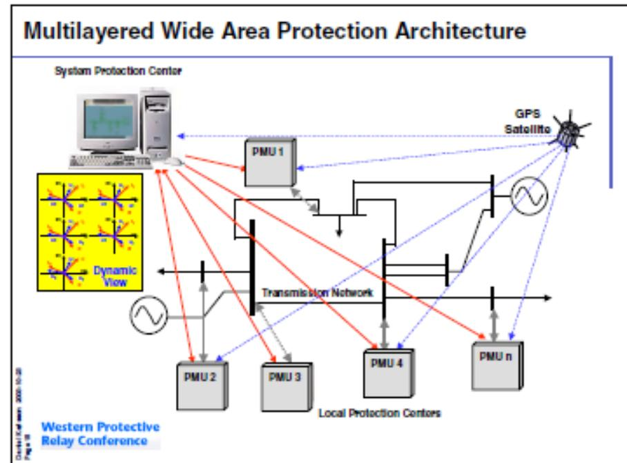
Figure 2: Multilayered wide area protection architecture 2
